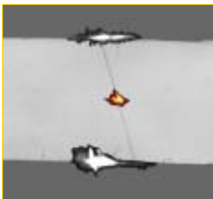
A scanning electron micrograph overlaid by an image of Rayleigh scattering from a carbon nanotube suspended across a 30 \mu\text{m} slit. (Courtesy: Feng Wang.)
