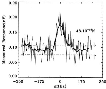
Fig. 1. The thin line is the response to an applied r.m.s. force of  $210 \times 10^{-18}$  N, averaged over 2560 traces. The signal is detected at a central frequency of 1.0156 MHz corresponding to a mode of the structure. The noise level corresponds to a minimum detectable force of  $48 \times 10^{-18}$  N with an intrinsic bandwidth of 80 Hz. The thick line is the smoothed trace.
